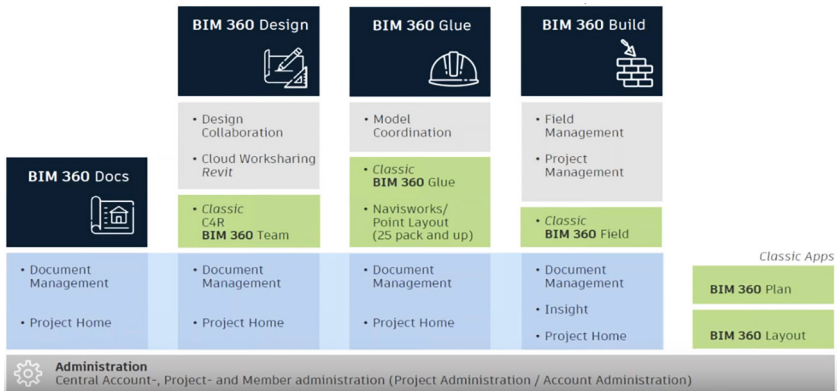
Fig. 4. Structure of the cloud platform BIM 360
